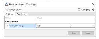
**2** Run the simulation. Note the effect of reduced voltage on the no-load speed.
