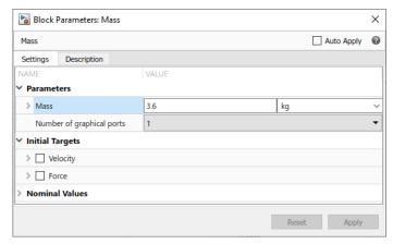
To specify the desired initial value for mass velocity, in the **Initial Targets** section, expand **Velocity**. The variable already has its **Priority** specified as **High**, which means that the solver will try to exactly satisfy this beginning value when it computes the initial conditions to determine the simulation starting point. Select the **Velocity** check box. In the **Value** field, type 10, then click **Apply**.
