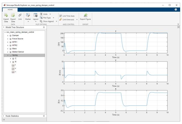
**3** Under the Spring node, select node x. The right pane displays the spring deformation data plotted over time.
